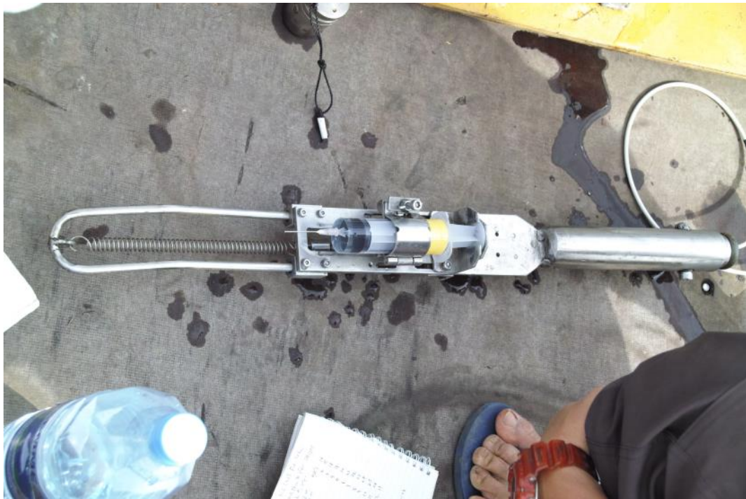
Fig 2. MK sampler. A plastic syringe filled with 10ml of 5M KOH solution is attached on the sampler.
